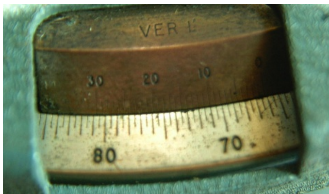
Figure 2: A photograph of the Vernier from the optical spectrometers used in the lab. The lighting isn't perfect but I would say the "0" of the Vernier scale is somewhere between the 66^{\circ}0' and 66^{\circ}30' marks (maybe a quarter of the way). The Vernier scale marks definitely appear to the left of the primary scale below 7' and probably to the right for marks above 12' (and the slight flaking and corrosion on the primary scale opposite the 13' , 14' , and 15' mark don't help in this judgement. Best line up is probably at 9' or 10' with an error of 2' . Giving an answer of 66^{\circ}9' or 66.15 \pm 0.03^{\circ} .
