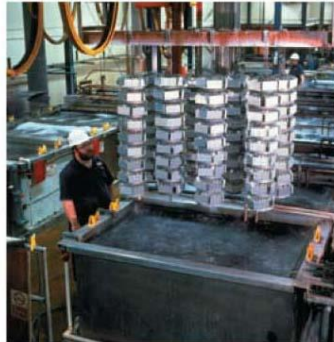
A rack of metal parts being lifted from the electrolyte solution after electroplating.
