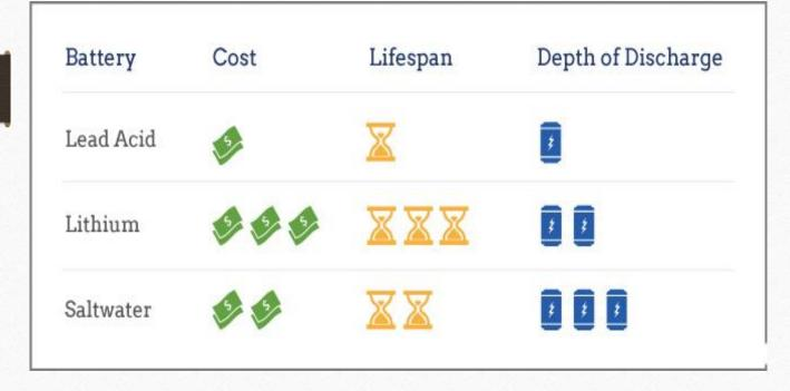
Depth of Discharge: How much energy can be cycled into and out of the battery in one cycle.
