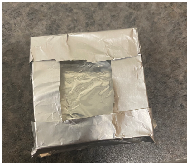
Figure 3.5: Scintillator partially wrapped in reflective foil.
