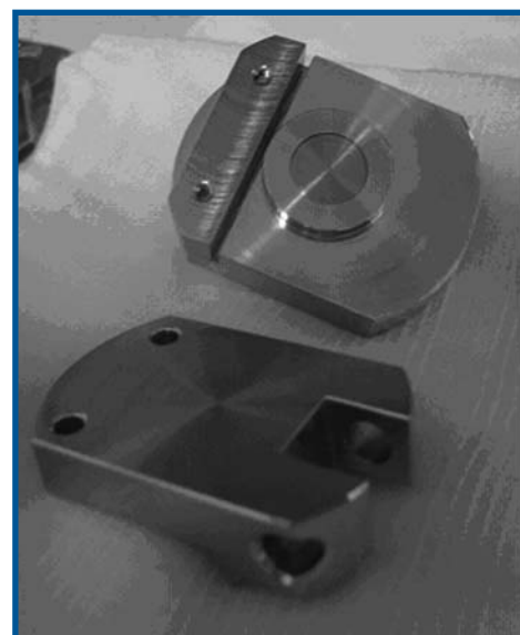
Fig. 2 Photograph of the sensor parts of the dilatometer of Figure 1. The upper piece contains the fixed circular plate, separated from the guard ring by the gap, which can be seen as the smaller circle. The lower piece is the moveable plate.
