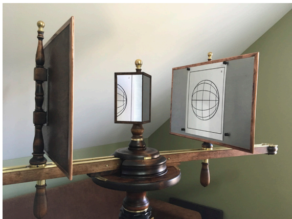
Fig. 16 Wheatstone Stereoscope. This is my second attempt at a stereoscope. It is in homage to Wheatstone's devices rather than a replica. The pivoting arms and circular forms are inspired by the idea of an orrery.
