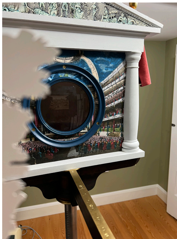
Fig. 9 Optical Theatre Lens. The inner lens (15 cm diameter; 60 cm focal length) can be removed and replaced with a larger lens (20 cm diameter; 90 cm focal length) that sits in the larger circular frame.
