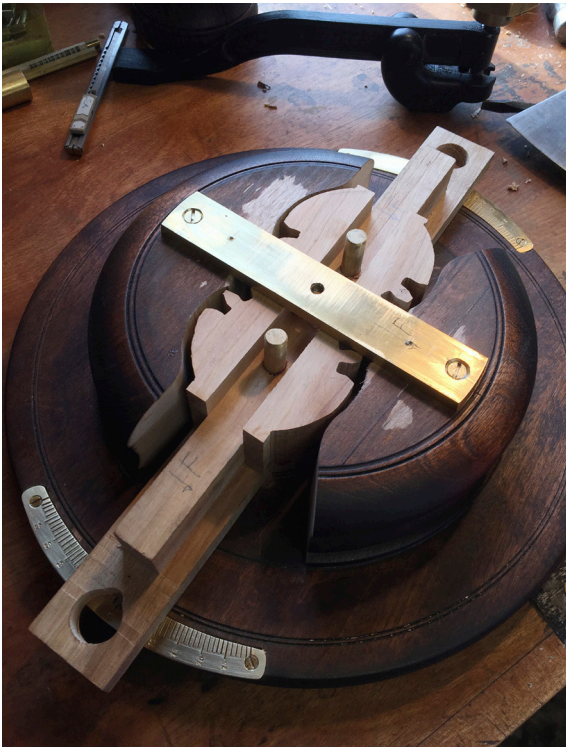
Fig. 14 Stereoscope Gears. These gears will synchronise the motion of the arms of the stereoscope, which have yet to be attached. Unlike Wheatstone's design (Fig. 13) there are two pivots here spaced at about the inter-ocular distance, so the angular measures more accurately reflect what is happening to the eyes.
