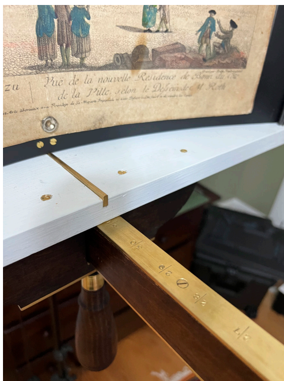
Fig. 10 Optical Theatre: Moveable Image Plate. Here you can see the track along which the image-plate can move and the adjusting handle below. You can also see how the image-plate can be curved or, by adjusting the knob at the back, be allowed to flatten again.
