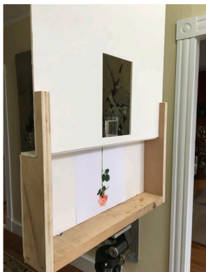
Fig.5 "Real Apparition" with Rose. The inverted image (left) is behind and below the window; the concave mirror (centre) stands behind that. From the front (right image) the projected illusion is of a flower placed in a vase.
