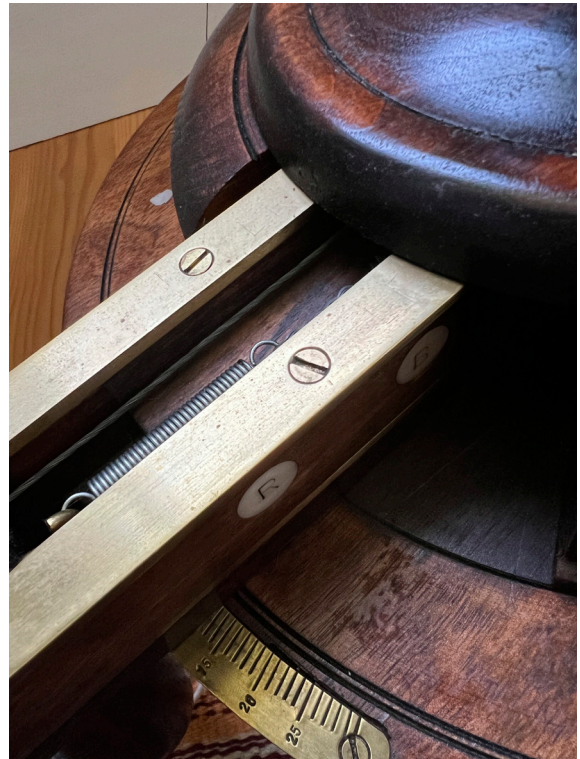
Fig. 15 Rigging Channel. The two image-plates are connected through the centre of the stereoscope by wires. When you pull or push one image-plate the other is pushed or pulled symmetrically. Note the "ivory" inlay on the side of the arm (made from deer antler rather than elephant tusk).
