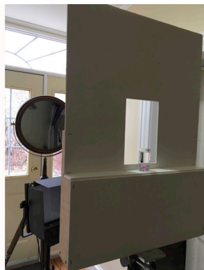
Fig.5 "Real Apparition" with Rose. The inverted image (left) is behind and below the window; the concave mirror (centre) stands behind that. From the front (right image) the projected illusion is of a flower placed in a vase.
