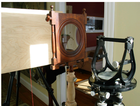
Fig. 11 Zogrscope Experiments. Here I have placed a laser pointer in the cradle of a theodolite to measure the refraction of light passing through an 18th-century zogrscope lens. I was able to calculate how this lens would affect the angle of convergence of the eyes when looking at a vue d'optique . That angle is greater when one looks at the centre of the vue than when one looks at the periphery. So, contrary to what 18th-century writers such as William Molyneux and Edmund Halley (1692) expect, the area that is often meant to be more distant (e.g. the back wall of a cathedral) should actually appear slightly closer.
