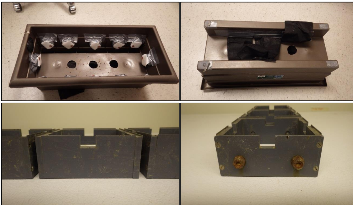
Figure 2.3: Top left – Exterior of the lightbox; top right – Interior of the lightbox; bottom right – End-on view of the settlement plate holder; and bottom left – Side-on view of the settlement plate holder.
