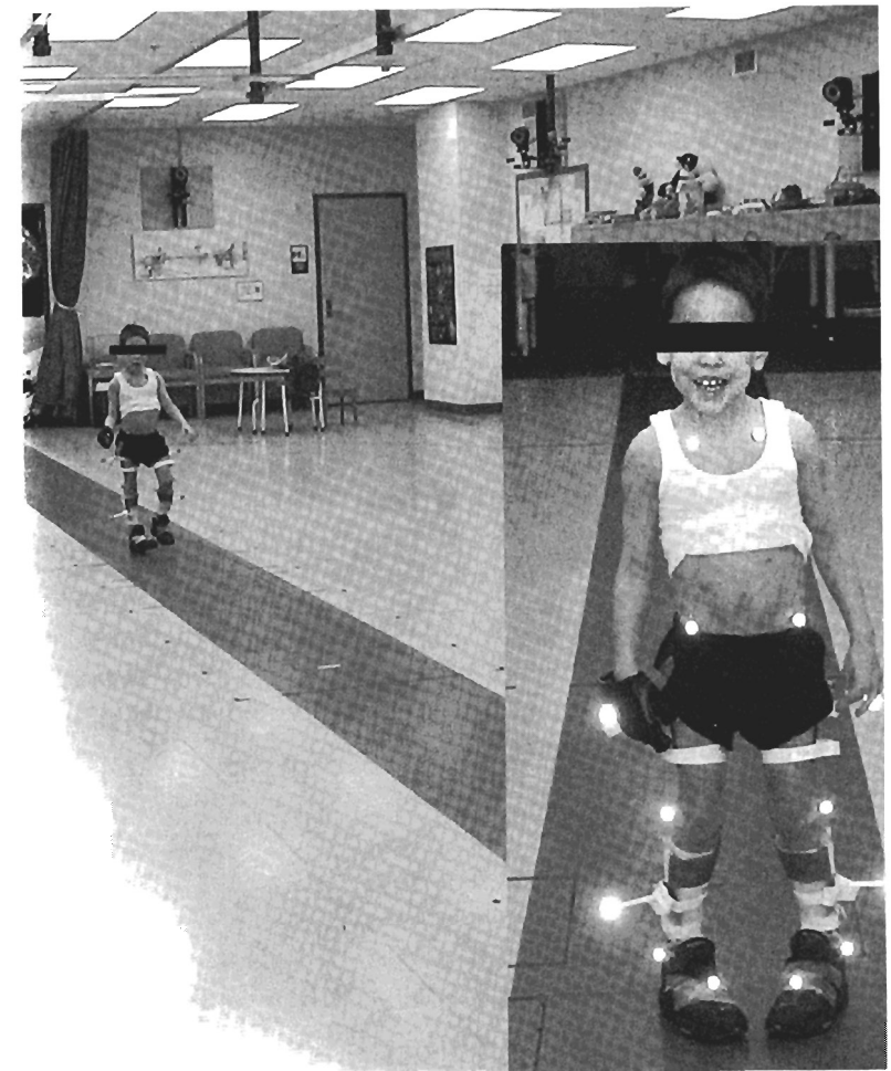
Figure 2.12 Gait assessment of a cerebral palsy patient in a clinical gait laboratory. Infrared cameras are mounted on the ceiling and walls to capture the reflected light from the spherical reflective markers mounted on both sides of the body. (Courtesy of the Gait Analysis Laboratory, Connecticut Children’s Medical Center, Hartford, CT.)
