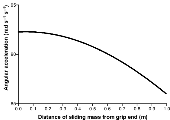
Figure 6 Angular acceleration values produced from the closed-form equation (using both gravitational and muscular torques) for each incremental shift of the sliding mass element along the club's shaft. The applied muscular torque was set at 20 Nm, and the club shaft was positioned at an angle of 20^\circ (i.e. \theta = 160^\circ in Fig. 1) above a horizontal line through the axis of rotation at the grip end.
