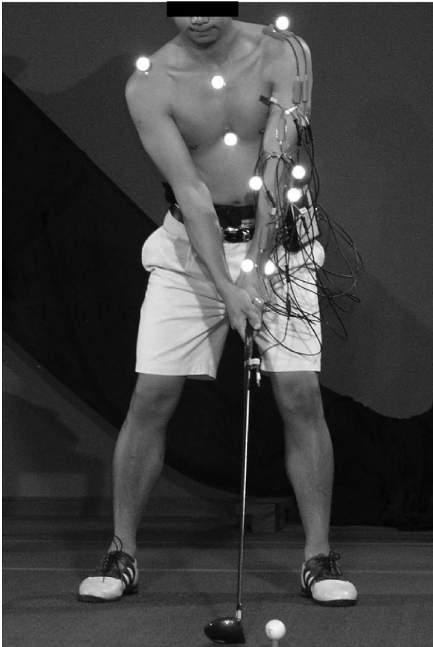
Fig. 2. Attachments of the EGMs and the markers.
