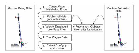
Figure 2: A block diagram of the processing done to extract 6 dof grip and club face kinematics from raw marker data.
