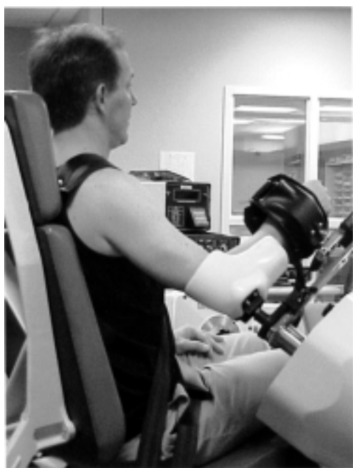
Fig. 1. Test subject immobilized in isokinetic testing device, upper limb in the test position of 45 degrees scapular plane abduction and the scapular neutral position.
